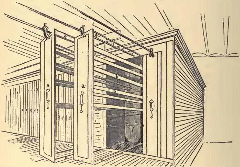
FIG. 57.—Superheating Chamber; Two Panels Drawn Open. a , Panels. (Two lower rack bars not shown.) b , Rack bars; c , rollers; d , iron bars connecting front and rear panels; e , rods upon which panels are suspended and travel; f , rear panel. Galvanized iron half-inch mesh screen in bottom of chamber.
